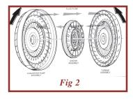
rotary motion theory, basically the normal oil path from the drive to the driven coupling member is redirected to the drive member in the same direction which helps the engine turn, hence torque multiplication. *Fig.* 2 The
