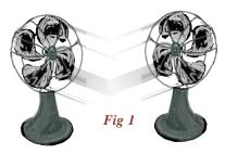
An example of a simple fluid coupling is to set two fans four inches apart facing each other and turn on one of them. *Fig.* 1 The air from the driving fan will impinge upon the
